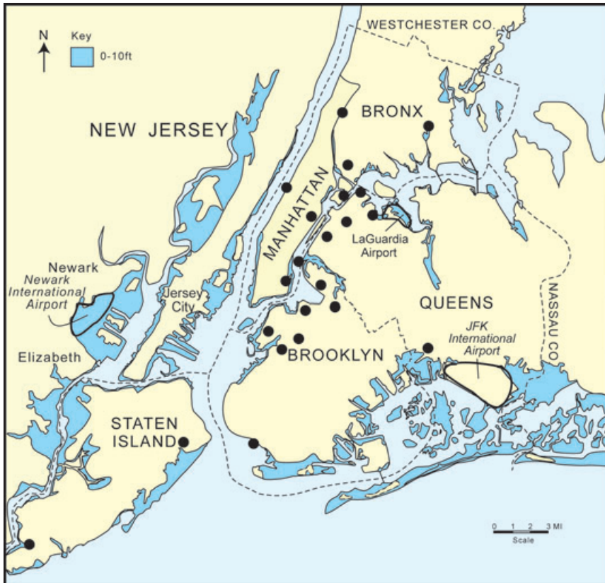
Figure 4.1. Locations of New York City power plants relative to 10-foot elevation contour.
